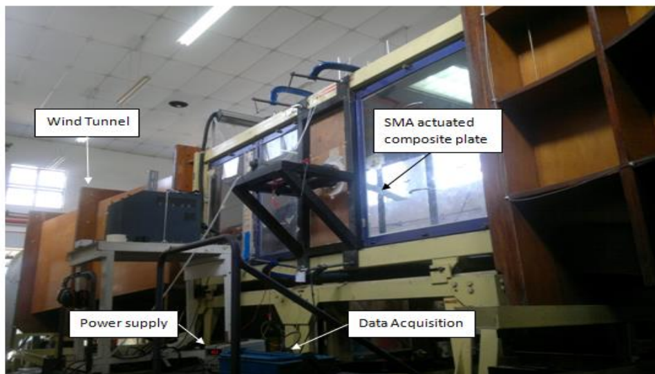
Figure 5. Wind tunnel experimental setup
