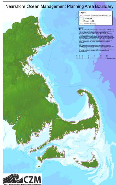
Figure 2. The line defines the landward limit of the Ocean Management Planning Area and represents the merger of a line projected 0.3 nautical miles from an approximate mean high water shoreline data set and closing lines digitized manually to ensure that most developed coastal embayments, ports, harbors, etc. are located landward of the nearshore boundary (MA Office of Coastal Zone Management).
