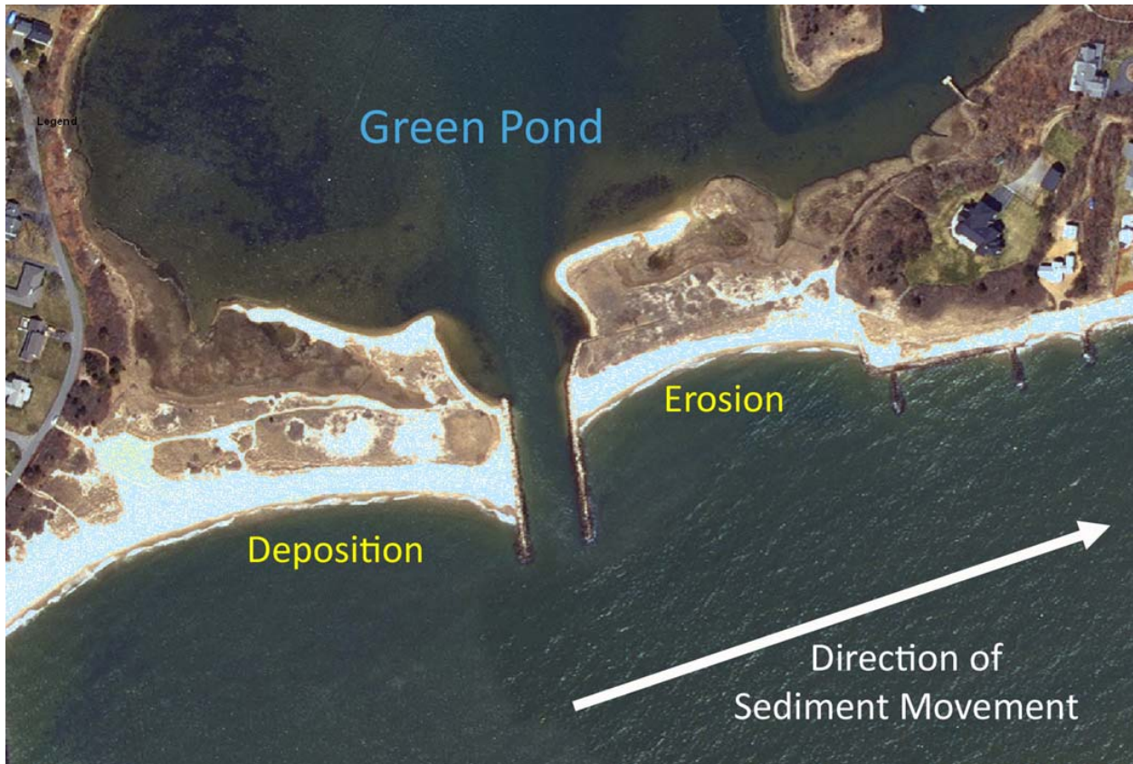
Figure 20: The areas where sediment is being deposited and eroded at the mouth of Green Pond.
