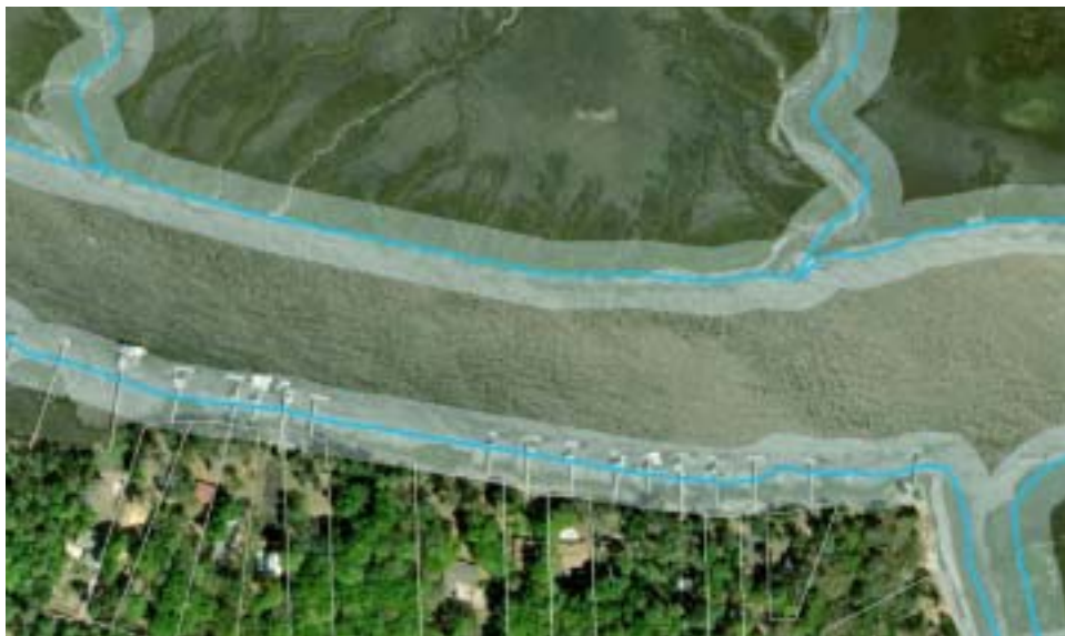
Figure 2.30: Buffering the water boundaries creates the ability to select parcels that intersect the buffered water layer.
