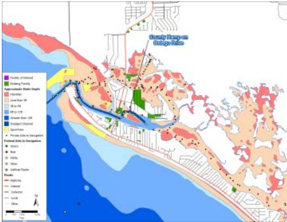
Figure 3.53: Water depth, existing sites and location of aids to navigation near the Ostego Drive ramp.
