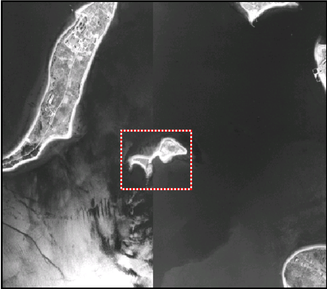
Figure 2.2. 1992 MassGIS composite orthophotograph shown with rectangular “Area of Interest” (AOI). The Rainsford Island AOI measures 835 m by 617 m and was created within ERDAS Imagine to subset extraneous data allowing for more efficient processing and analysis. The same AOI was also used to subset and reduce other image data utilized within this study. The figure also shows why it was necessary to mosaic many of the MassGIS orthophotographs together. The Island, though relatively small, was often divided into two separate files which can be seen by the tonal difference between the left and right side of this image.
