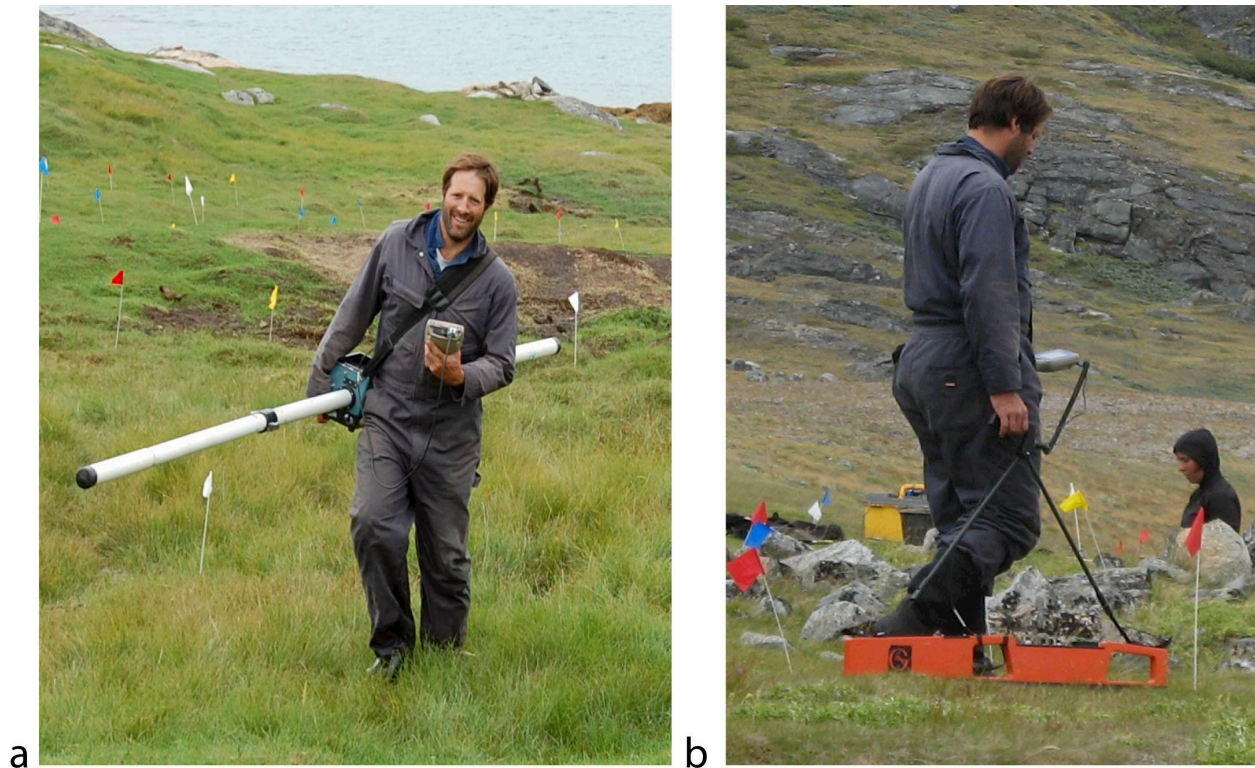
Figure 3. Electromagnetic surveying with (a) the Geonics EM-31 and (b) the Geonics EM-38.
