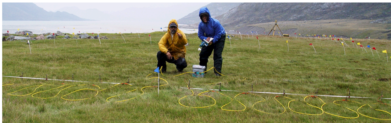
Figure 7. Electrical resistivity surveying with Syscal Kid meter.
