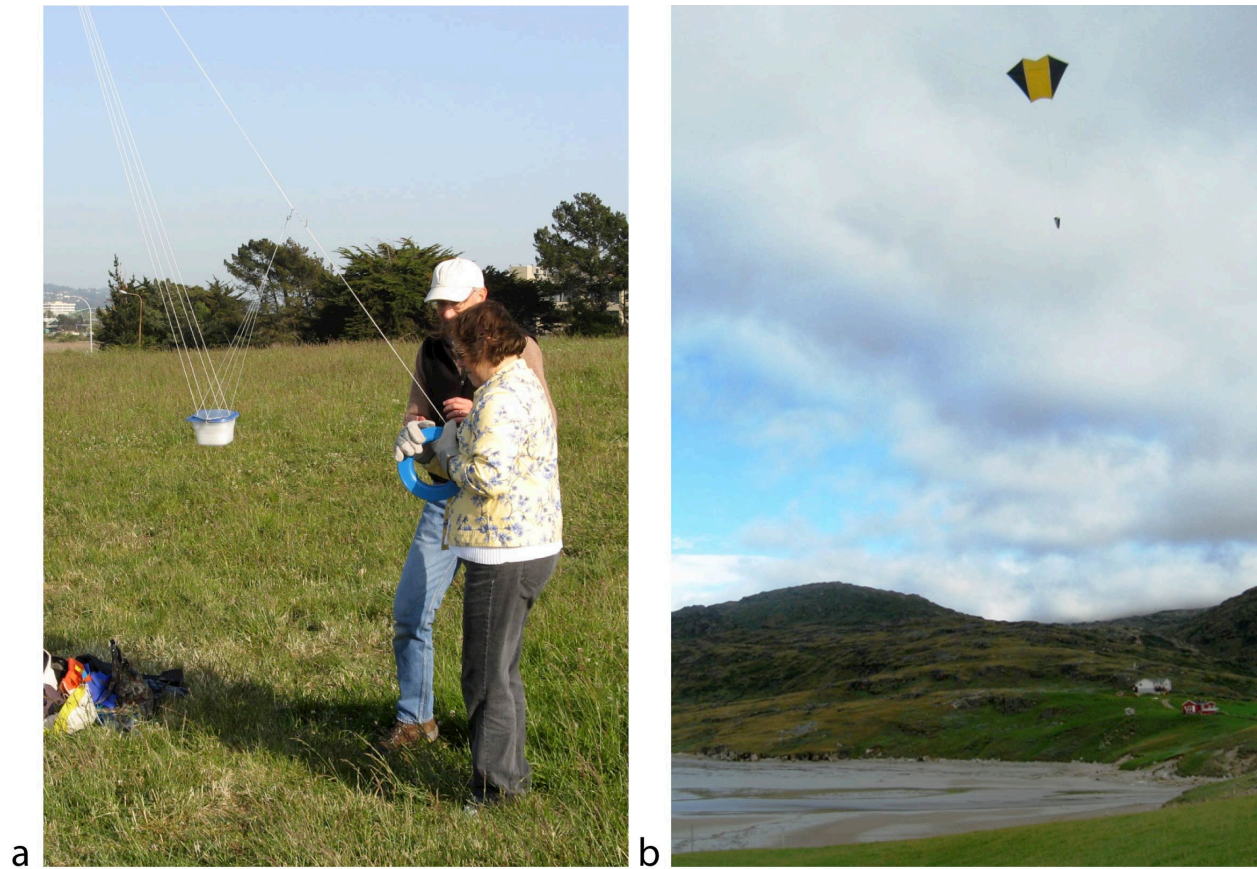
Figure 2. Kite-based aerial photography: (a) KAP box and Picavet string suspension, and (b) kite in flight at Ø66.
