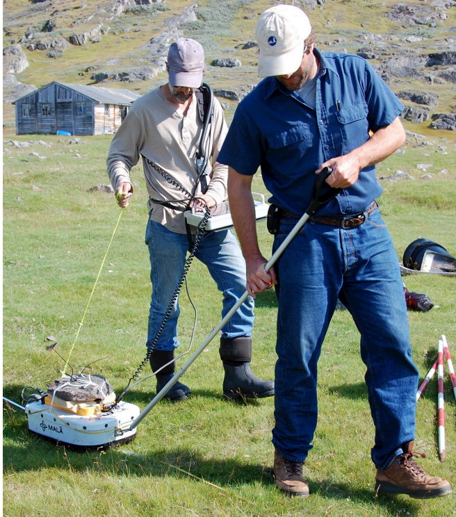
Figure 11. GPR surveying with the Malå unit equipped with the 500 MHz antenna.
