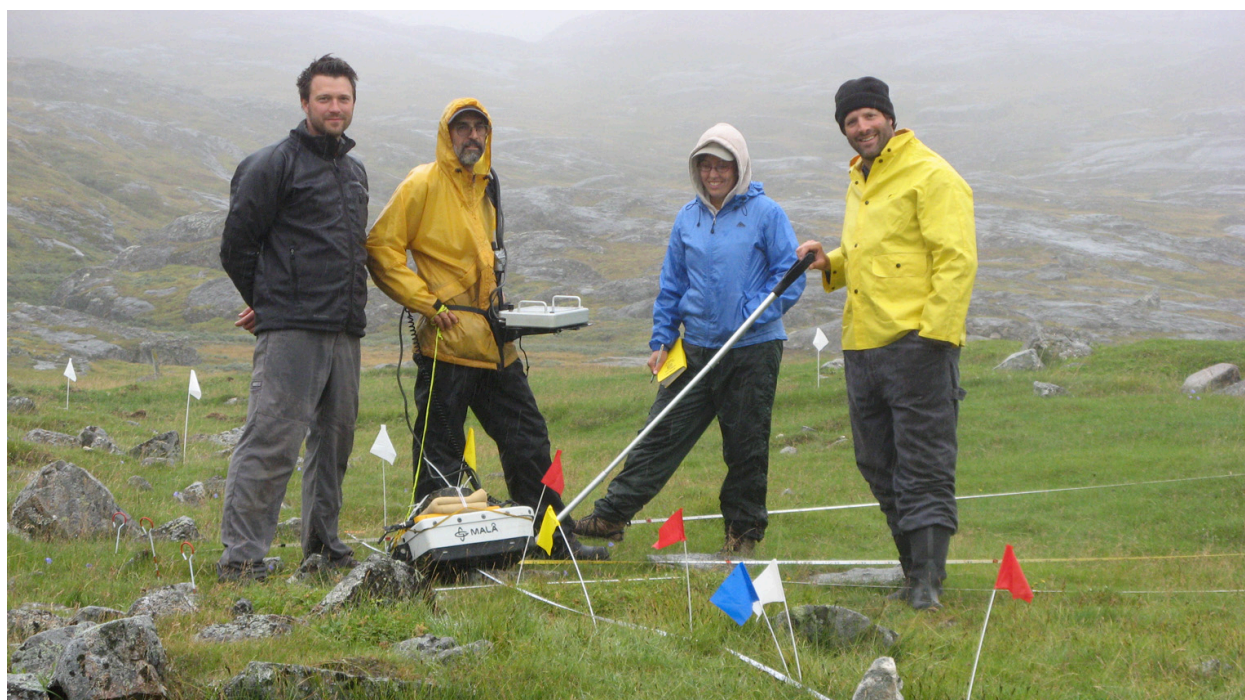
Figure 15. GPR antenna elevated off ground surface by rocks.
