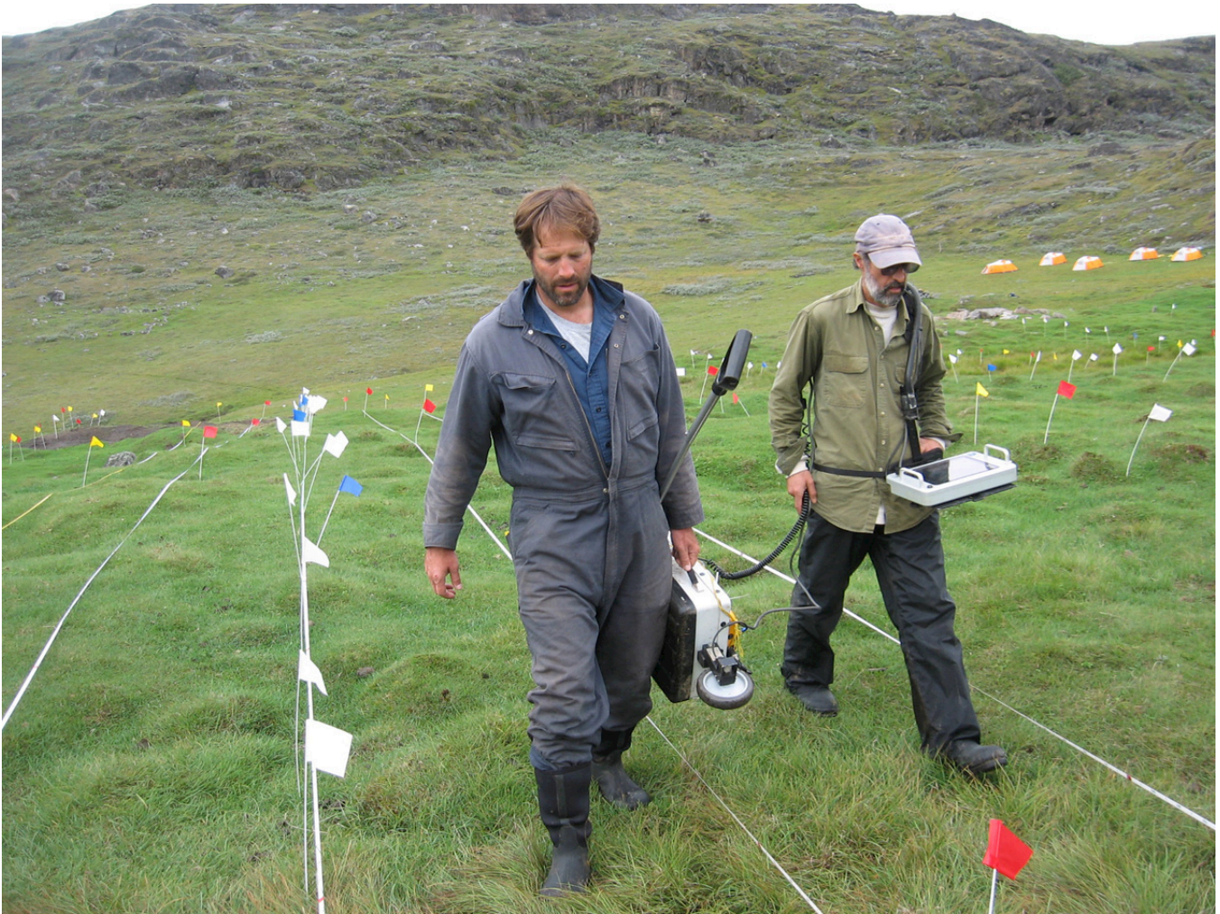
Figure 40. Ø172 GPR surveying with the Mala unit equipped with 500 MHz antenna.
