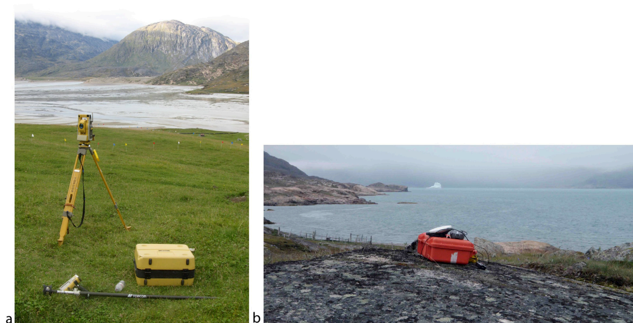
Figure 1. Survey grid establishment: (a) GPT9005A robotic total station, and (b) Trimble GeoXH GPS with a Zephyr antenna.
