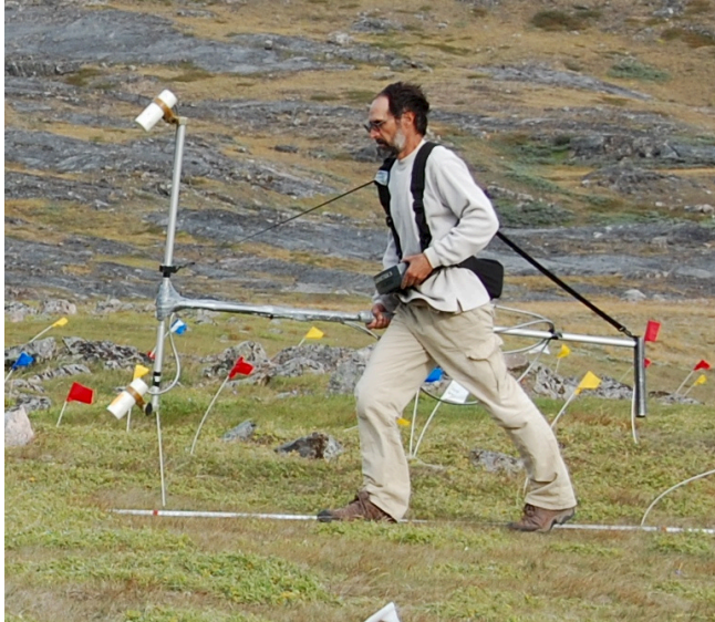
Figure 9. Magnetic surveying with the Geometrics G-858 cesium-vapor gradiometer.
