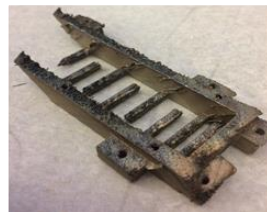
Figure 5. Fabricated bandpass filters with (a) line supports and minimal support surface, and (b) point supports with minimal support surface and z-height.
