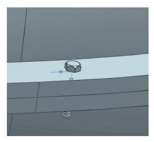
> Repeat the same procedure to add bolts and nuts to all the holes in the casing.
