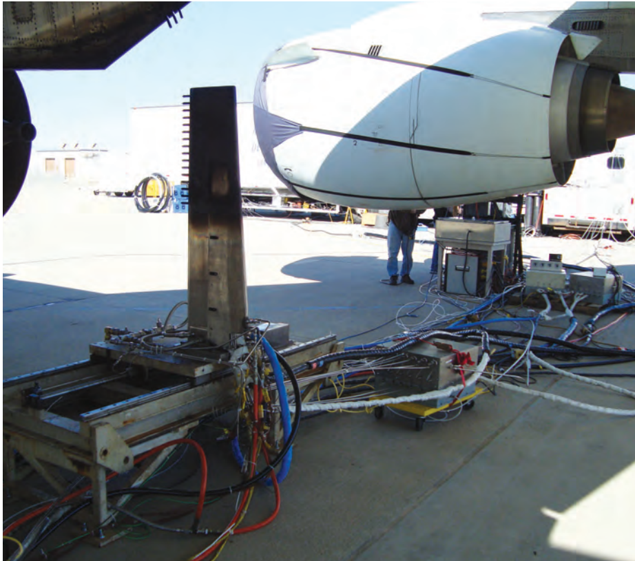
Using equipment that captures and measures exhaust, the researchers tested biofuels in the same type of engine used by a Boeing 737.
