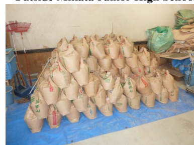
Produced pellets (One bag is about 10kg = quantity used by one stove to operate for one day)
