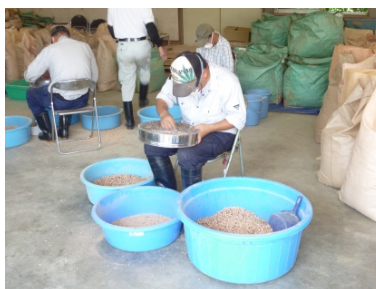
A pellet production factory in the town (Pellets are sifted after production to obtain pellets of uniform size)
