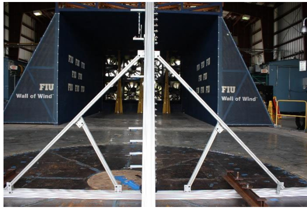
Figure 8. Measurement of wind velocity profile for open terrain.
