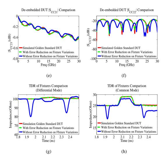
Figure 18. DUT comparisons between golden standard and de-embedded results: (a) |SDD11|; (b) |SDD21|; (c) |SDD22|; (d) |SCC11|;: (e) |SCC21|; (f) |SCC22|;(g) differential mode TDR characteristic impedance; (h) common mode TDR characteristic impedance.(cont.)
