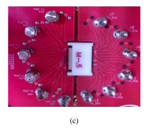
Figure 9. The layout and the manufactured test coupon: (a) Total (DUT embedded in between the fixtures) layout; (b) 2X-Thru fixture layout with exact spider legs like design as the Total; (c) manufactured Total.(cont.)
