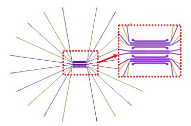
Figure 14. A better 2X-Thru calibration pattern.
