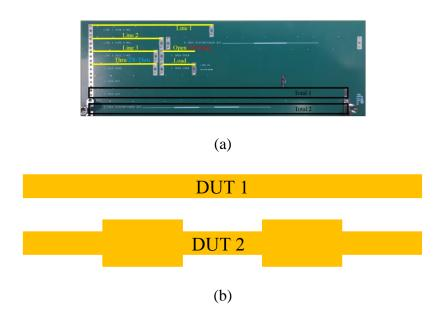
Figure 9. (a) A manufactured test coupon, with calibration patterns for TRL (highlighted in yellow), 2X-thru (highlighted in blue) and 1X-reflection (highlighted in red).
