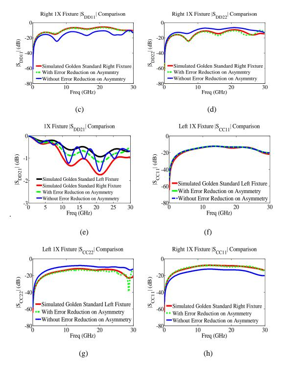
Figure 15. Fixture characterization result comparisons: (a) |SDD11| of left 1X fixture; (b) |SDD22| of left 1X fixture; (c) |SDD11| of right 1X fixture; (d) |SDD22| of right 1X fixture; (e) |SDD21| of 1X fixture; f) |SCC11| of left 1X fixture; (g) |SCC22| of left 1X fixture; (h) |SCC11| of right 1X fixture; (i) |SCC22| of right 1X fixture; (j) |SCC21| of 1X fixture. (cont.)
