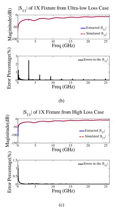
Figure 6.  $|S_{11}|$  comparison and error percentage of fixture from (a) lossless; (b) ultra-low loss; and (c) high loss. (cont.)
