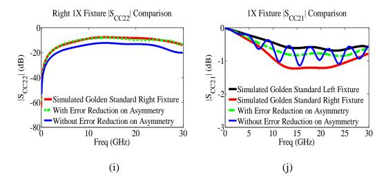
Figure 15. Fixture characterization result comparisons: (a) |SDD11| of left 1X fixture; (b) |SDD22| of left 1X fixture; (c) |SDD11| of right 1X fixture; (d) |SDD22| of right 1X fixture; (e) |SDD21| of 1X fixture; f) |SCC11| of left 1X fixture; (g) |SCC22| of left 1X fixture; (h) |SCC11| of right 1X fixture; (i) |SCC22| of right 1X fixture; (j) |SCC21| of 1X fixture. (cont.)
