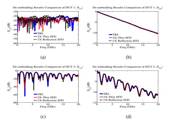
Figure 10. De-embedded results comparison: (a)  $|S_{11}|$  of DUT 1; (b)  $|S_{21}|$  of DUT 1;  $|S_{11}|$  of DUT 2;  $|S_{21}|$  of DUT 2.
