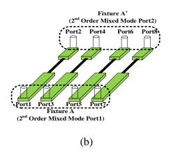
Figure 4. An example of 2X-Thru calibration standard of a 2<sup>3</sup>-port network: (a) 1st order mixed-mode; (b) 2nd order mixed-mode.
