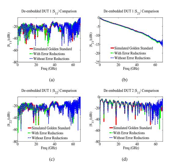
Figure 21. DUT comparisons on the IEEE P370 test coupons between golden standard and de-embedded results: (a) |S11| of DUT 1; (b) |S21| of DUT 1; (c) |S22| of DUT 1; (d) |S11| of DUT 2; (e) |S21| of DUT 2; (f) |S22| of DUT 2;(g) TDR characteristic impedance of DUT 2; (h) TDR characteristic impedance of DUT 2.
