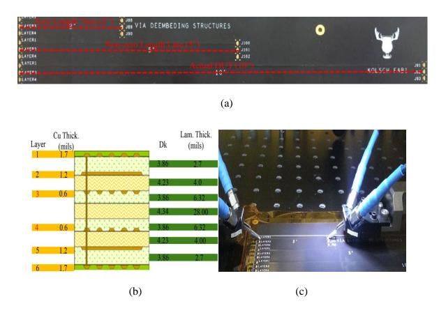
Figure 10. (a) A test coupon with marked TLD standards; (b) stack up information of the test coupon; (c) GSSG microprobes are used in the measurement.
