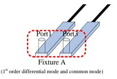
Figure 6. Example of a two-port 1X-reflection calibration pattern.
