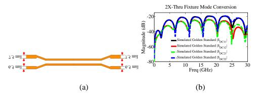
Figure 7. 2X-Thru with unbalanced design: (a) upper trace and lower trace has different width of lead-in portion; (b) mode conversion terms.
