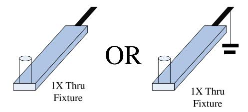
Figure 1. 1X-Reflection SFD calibration patterns.
