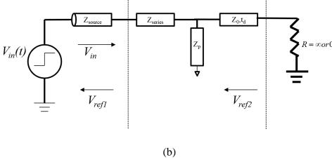
Figure 5. A transmission line in between discontinuity and termination in the 1X-Reflection fixture design (a) design requirement; (b) reflected waveforms from discontinuities.
