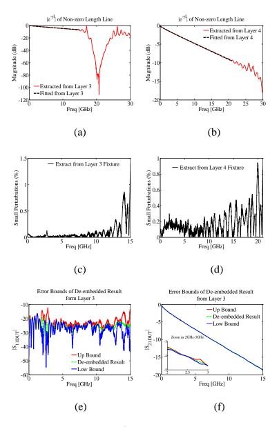
Figure 11. (a) Extracted and fitted  $|e^{\gamma l}|$  from case C; (b) extracted and fitted  $|e^{\gamma l}|$  from case D; (c) small perturbations of  $|e^{-\gamma l}|$  from case C; (d) small perturbations of  $|e^{-\gamma l}|$  from case D; (e) error bounds of  $|S_{11}|$  from case C; (f) error bounds of  $|S_{21}|$  from case C; (g) Error bounds of  $|S_{11}|$  from case D; (h) error bounds of  $|S_{21}|$  from case D.
