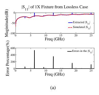
Figure 6.  $|S_{11}|$  comparison and error percentage of fixture from (a) lossless; (b) ultra-low loss; and (c) high loss.
