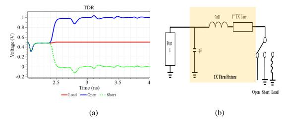
Figure 4. An example of TDR response from s-parameter input: (a) 1X-reflection TDR response with SOL terminations; (b) the corresponding 1X-reflection circuit diagram.
