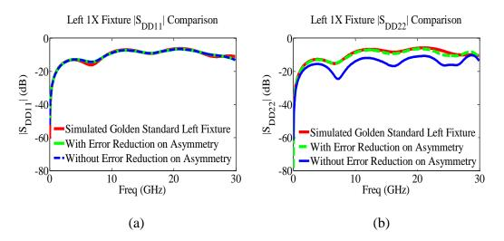
Figure 15. Fixture characterization result comparisons: (a) |SDD11| of left 1X fixture; (b) |SDD22| of left 1X fixture; (c) |SDD11| of right 1X fixture; (d) |SDD22| of right 1X fixture; (e) |SDD21| of 1X fixture; (f) |SCC11| of left 1X fixture; (g) |SCC22| of left 1X fixture; (h) |SCC11| of right 1X fixture; (i) |SCC22| of right 1X fixture; (j) |SCC21| of 1X fixture.
