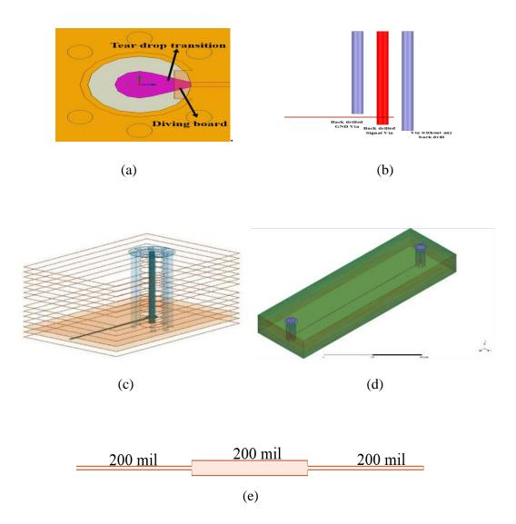
Figure 8. (a)Top view of case A; (b) side view of case A;(c) the half of zero length Thru standard; (d) non-zero length Line standard; (e) DUT embedded in the Total.
