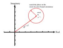
Figure 7. Complex errors combinations of  $e^{-\gamma l}$ .
