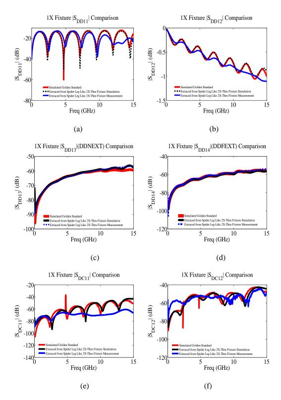
Figure 11. 1X fixture electrical performance comparisons: (a) |SDD11|; (b) |SDD12|; (c) |SDD13| (NEXT); (d) |SDD14| (FEXT); (e) |SDC11|;(f) |SDC12|;(g) |SDC13|;(h) |SDC14|.
