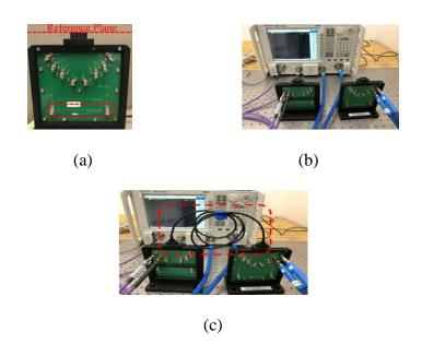
Figure 13. (a) 1X-Reflection SFD calibration board; (b) 1X-Reflection measurement for left and right fixtures; (c) the measurement of Total.
