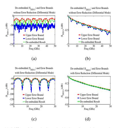
Figure 19. Differential mode de-embedded results and the error bounds: (a) |SDD11|without enforcing the error reductions; (b) |SDD21|without enforcing the error reductions; (c) |SDD11| with enforcing the error reductions; (c) |SDD21| with enforcing the error reductions.
