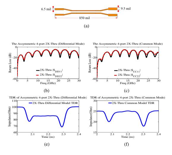
Figure 14.The asymmetric  $2^2$ -port 2X-Thru: (a) full-wave models; (b)  $|S_{DD11}|$  and  $|S_{DD22}|$  comparison; (c)  $|S_{DD11}|$  and  $|S_{DD22}|$  comparison; (d) differential mode TDR impedance comparison; (e) common mode TDR impedance comparison.
