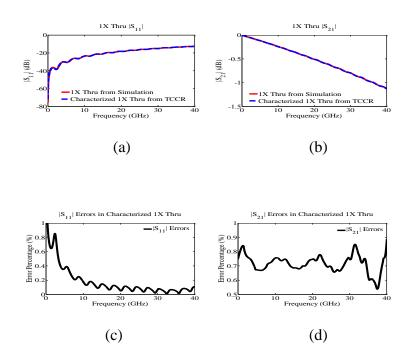
Figure 8. Fixture characterization results verification: (c) Error percentage of  $|S_{11}|$ ; (d) Error percentage of  $|S_{21}|$ .
