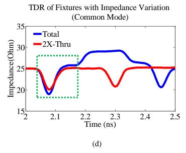
Figure 17. Fixture impedance variations between 2X-Thru and Total: (a) 850 mil symmetric 2X-Thru; (b) 1350 mil Total with the impedance variations at lead-in traces; (c) 5 Ohm differential characteristic impedance differences at lead-in traces of fixtures; (d) 1.5 Ohm common characteristic impedance differences at lead-in traces of fixtures.(cont.)
