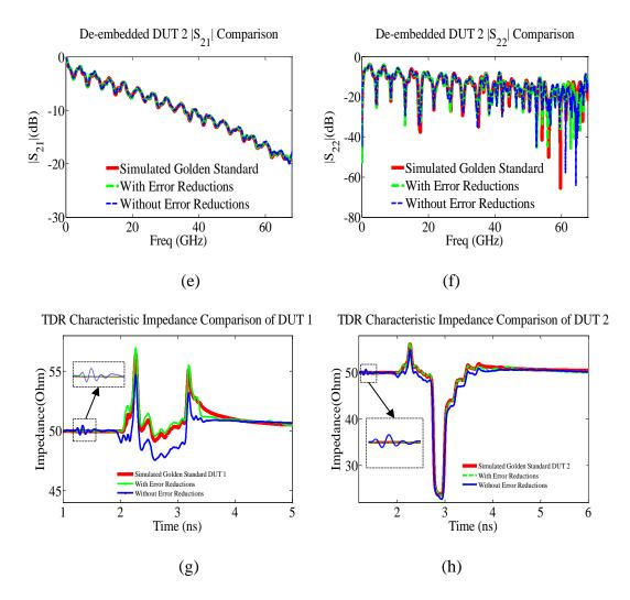
Figure 21. DUT comparisons on the IEEE P370 test coupons between golden standard and de-embedded results: (a) |S11| of DUT 1; (b) |S21| of DUT 1; (c) |S22| of DUT 1; (d) |S11| of DUT 2; (e) |S21| of DUT 2; (f) |S22| of DUT 2;(g) TDR characteristic impedance of DUT 2; (h) TDR characteristic impedance of DUT 2.(cont.)
