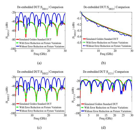
Figure 18. DUT comparisons between golden standard and de-embedded results: (a) |SDD11|; (b) |SDD21|; (c) |SDD22|; (d) |SCC11|;: (e) |SCC21|; (f) |SCC22|;(g) differential mode TDR characteristic impedance; (h) common mode TDR characteristic impedance.
