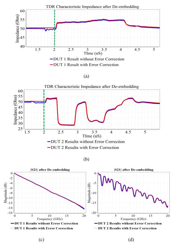
Figure 12. TDR characteristic impedance results of 1X-reflection de-embedding with and without the fixture error correction: (a) DUT 1; (b) DUT 2; (c) DUT 1; (d) DUT 2.
