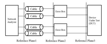
Figure 2. A typical de-embedding diagram
