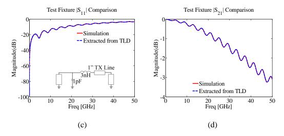
Figure 5. (a) Non-zero length Line  $|e^{\gamma l}|$  comparison; (b) Non-zero length Line transmission phase comparison; (c) Fixture A  $|S_{11}|$  comparison (schematic is embedded); (d) Fixture A  $|S_{21}|$  comparison.(cont.)
