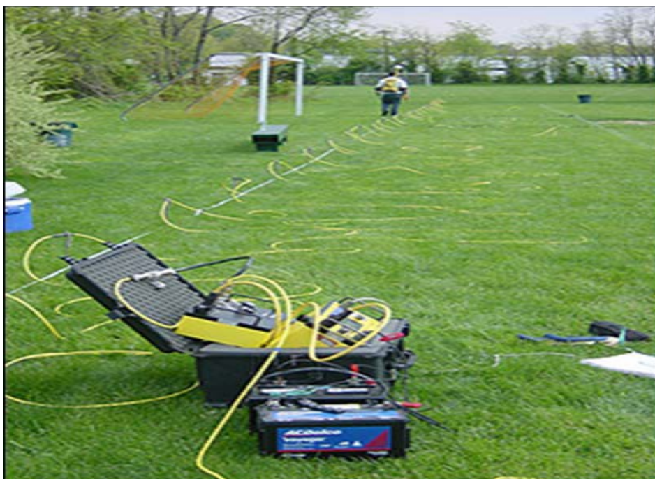
Figure 5.6. The field equipment of the ERT.
