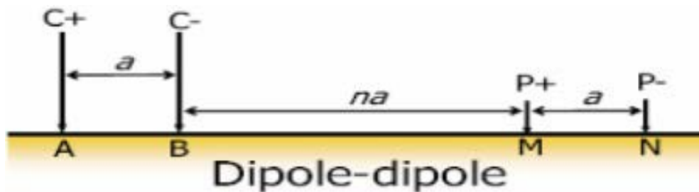
Figure 5.4. Dipole-dipole electrode array.
