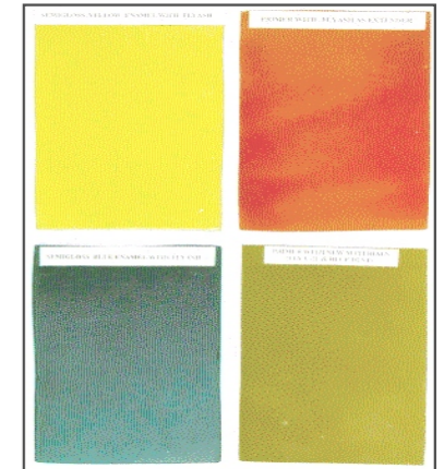
Fly ash paint coated on MS steel plate
