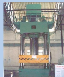
Hydraulic Press 400 tonnes
