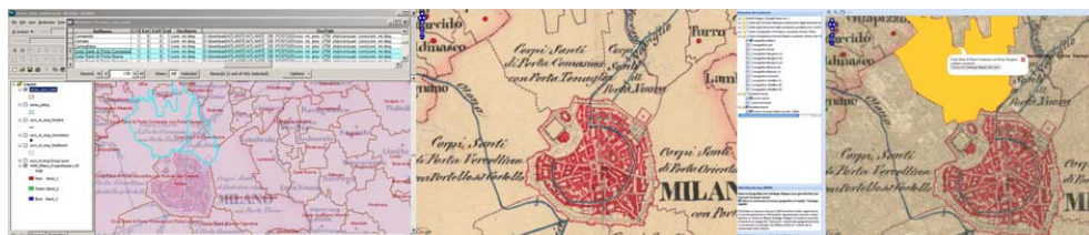
Figure 3: (Left) Extraction of Map Sheets Belonging to Ancient Municipalities' Extensions in the 19th Century, through a Vector File. (Far Left) Classified with respect to the Name of Census Parcel Units, using a WPS Tool. (Right) Direct Comparison to the Current Vector File in the Geographic Navigation
