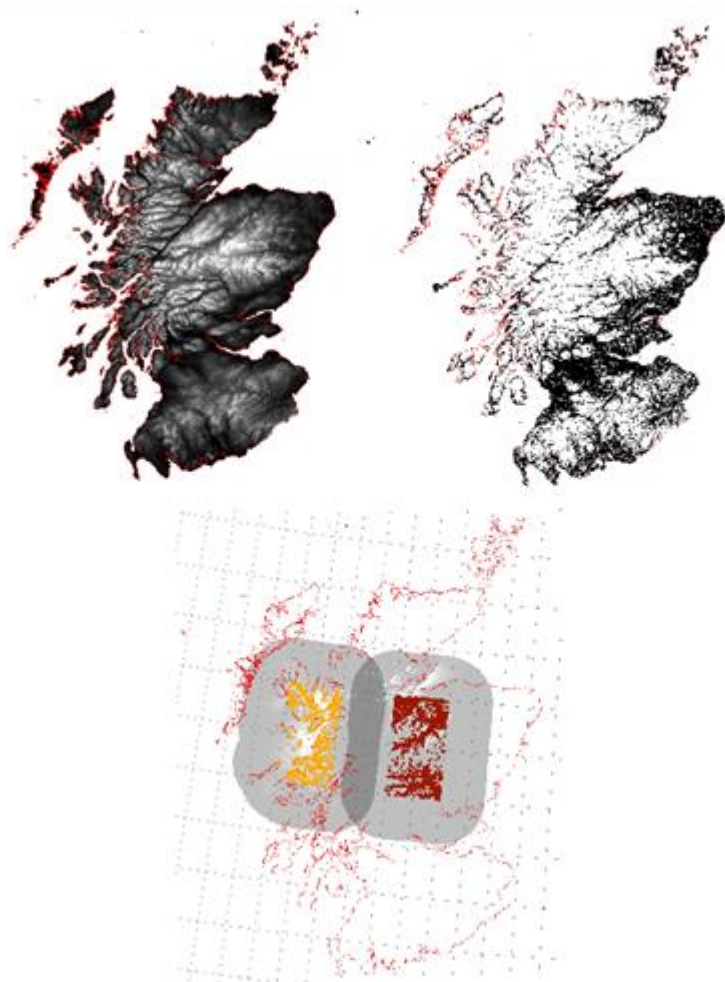
Figure 2 a) The Digital Elevation Model for Scotland. b) The buildings layer from the Ordnance survey. c) Example of the division of the buildings layer by latitude and longitude and the generation of the buffered overlay.
