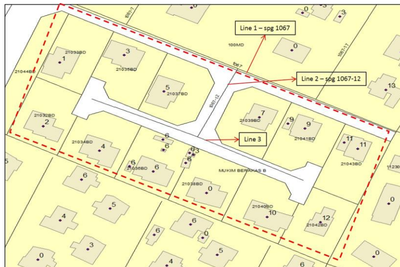
Figure 7: Sample of Access Road (Line 2) that Act as Merger to Two Road Segments (Line 1 and Line 3). Its Attribute Value 'Spg 1067-12' is used for All Addresses within the Dotted Block. Addresses inside the Dotted Block are obtained from Stage 1 and Visually They Are Based on Line 3.
