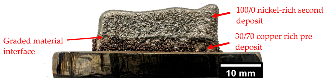
Figure 9. Copper–nickel FGM deposit fabricated with 30/70 as the pre-deposit and 100/0 as the second deposit. The set 3 duty cycle rampdown parameter was used at the dissimilar material interface.
