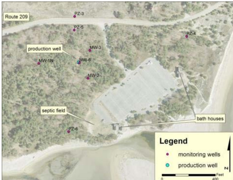
Figure F-2. Map of the well field and park infrastructure at Popham Beach State Park, showing the production pumping well and monitoring well locations. Aerial photograph from 2013.
