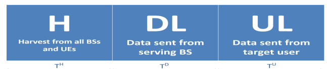
FIGURE 2. Time slot partitioning to include EH slot.
