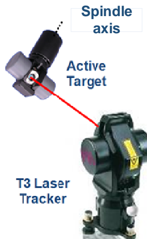
Figure 8: Illustration of laser tracker and active target.
