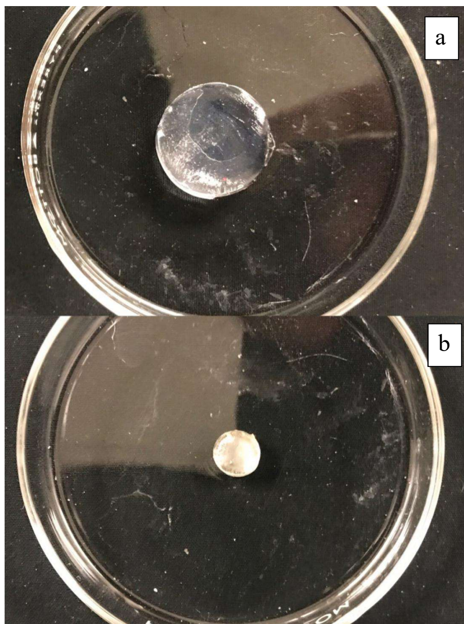
Figure 3.2 Presentation of (a) the gel disk in a fully swollen state and (b) gel in the dry state
