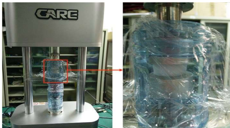
Figure 2.11 The uniaxial static compression test with the electromagnetic dynamic mechanical test system. (Zhang et al., 2017)
