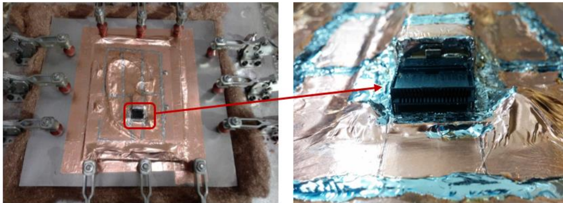
Figure 3.12 A Close View of FQSFP Connector in the Measurement Setup
