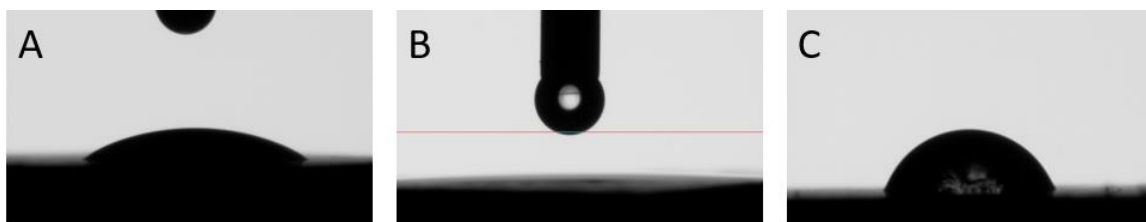
Figure S2. (a) Diiodomethane contact angle on heated LCO showing a 20^\circ decrease as compared to as-received LCO. Comparison of water droplet contact angles on (b) heated LCO surface and (c) as-received LCO surface.
