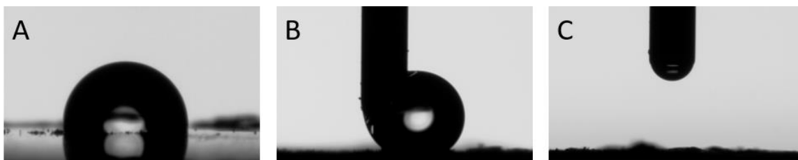
Figure S5. (a) Water droplet on the hydrophobic graphite surface. (b) Water droplet showing the hydrophobicity of as-received C65. (c) Water droplet soaking through treated C65, showing a change to hydrophilicity.
