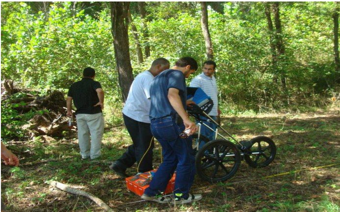
Figure 4.7. Acquisition of GPR Data
