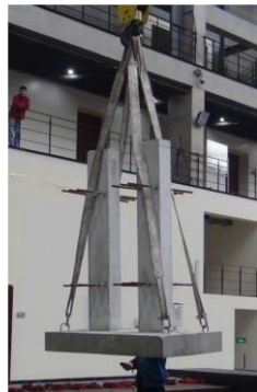
(e) Pier placement on shake table
