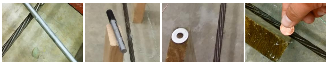
Figure 3.3. Four objects tapped on the test strand to create different acoustic noises
