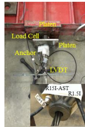
(c) Anchorage detail (load cell)
