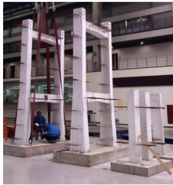
(c) Bridge towers and piers after curing
