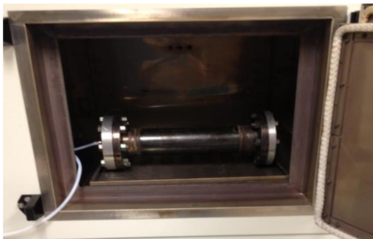
Figure 9. Chamber setup used for argon aging
