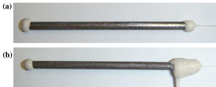
Figure 5.4. Steel tube encapsulated OP: (a) before and (b) after copper wire connection.
