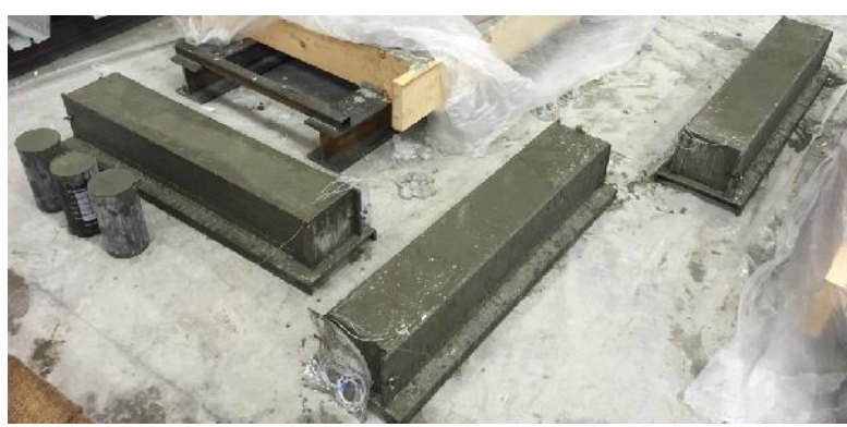
Figure 7.3. RC beams and cylinders for corrosion test.
