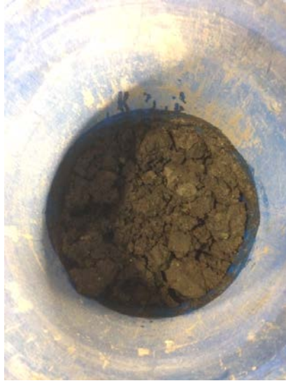
Figure C.1- Flash setting of the unsuccessful mix (FA Type 1)
