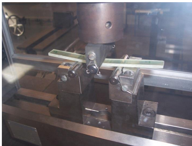
Figure 5.7. Flexure test setup
