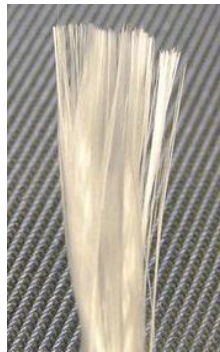
Figure 2.1. Conventional E-glass fibers manufactured by Owens Corning
