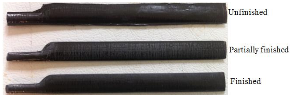
Figure 3.5 Manufactured composite blades
