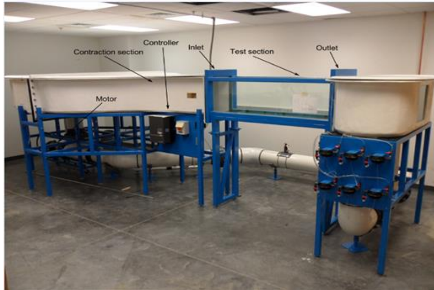
Figure 3.1. Water tunnel facility
