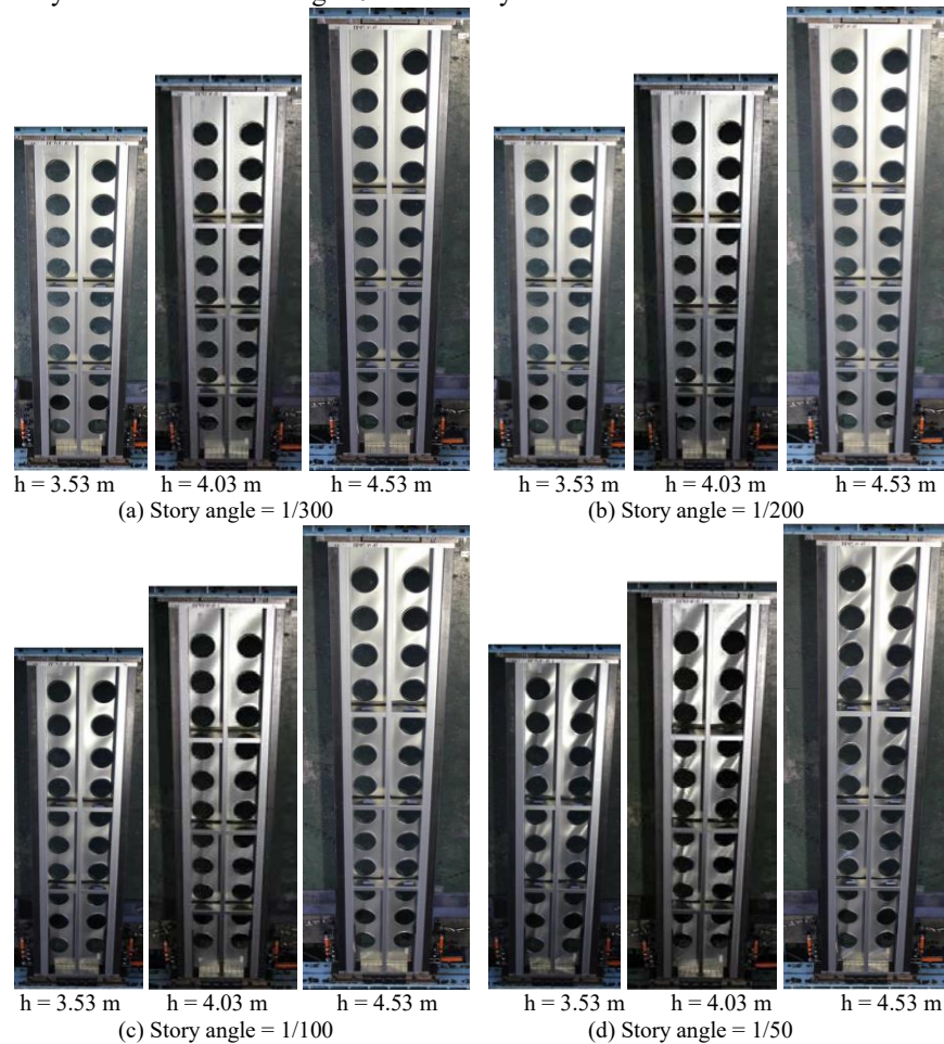
Figure 20: Photos of walls at story angles of 1/300~1/50 by shear experiments
