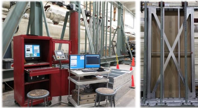
Figure 1 – Shear Wall Test Setup and strap-braced shear wall with gypsum panel
