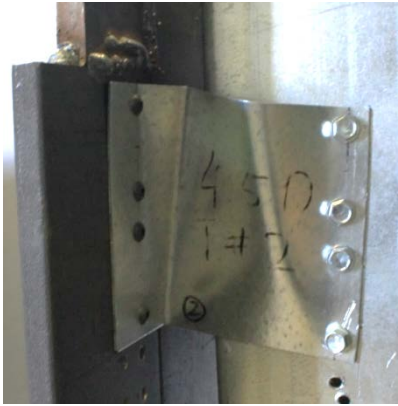
Figure 7 - Failure mode of shear test II4.5 #b2
