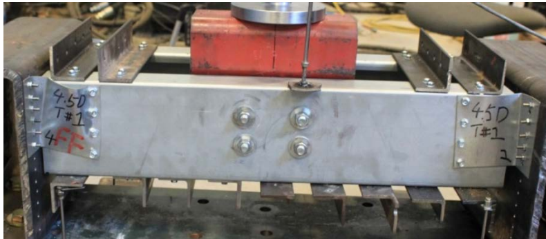
Figure 6 - Failure mode of joist 4.5D T#1
