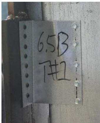
Figure 10 - Failure mode of shear test II6.5 #1
