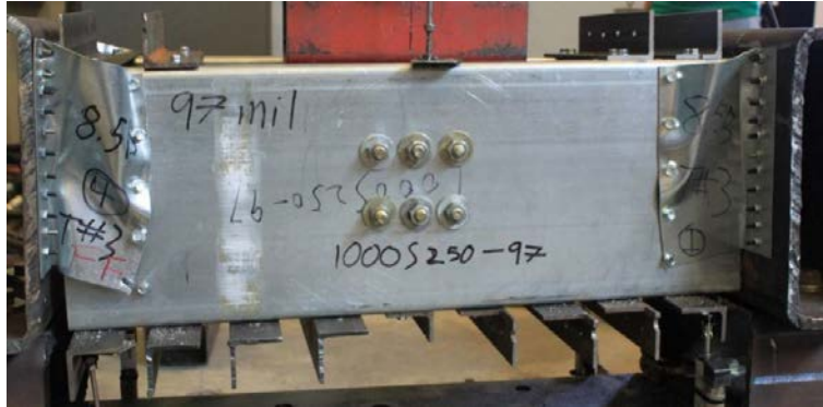
Figure 13 - Failure mode of 8.5B T#3
