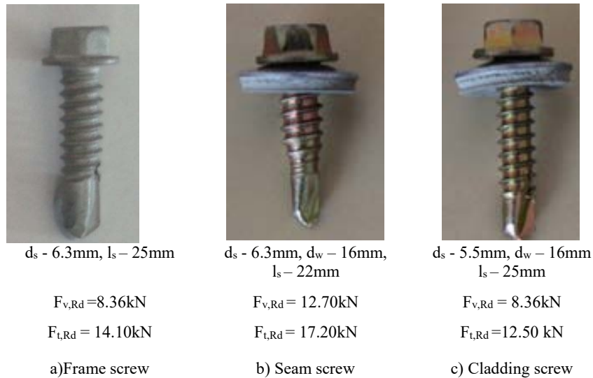
Figure 3 Dimensions and mechanical properties of screws
