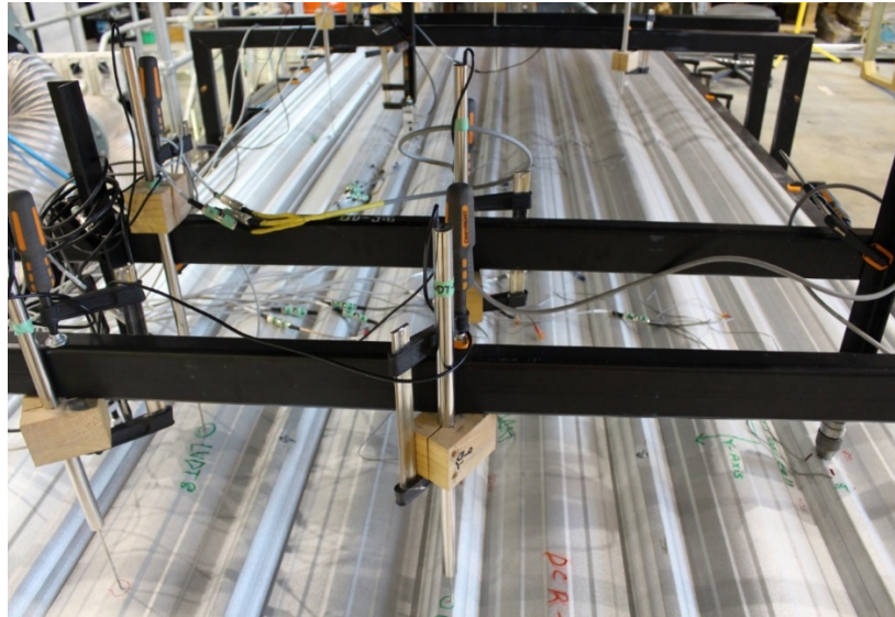
Figure 7: Deflected shape of the drap curved roof cladding (DCR-S800-t0.55)
