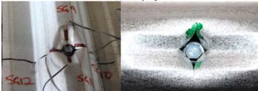
(b) Splitting failure
