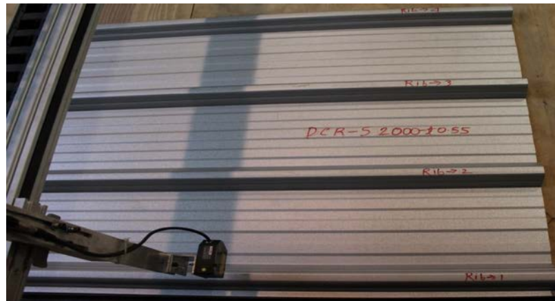
(b) Photograph of imperfection measuring setup
