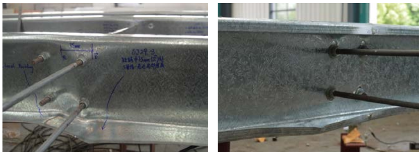
Figure 6. Failure modes of Z-purlin and C-purlin with one row of sag rods
