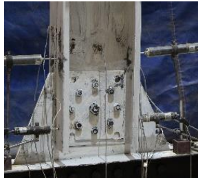
CB connection with 2mm S-beam
