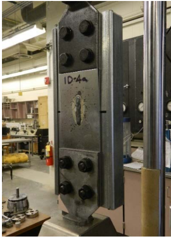
Figure 2. Typical slot weld test specimen, consisting of a 14 gage sheet slot welded to a 16 gage sheet, mounted in the bracing jig and installed in a 20 kip (89 kN) MTS testing machine.
