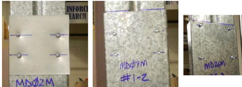
Figure 6. Photograph showing specimen with 14 GA plate, 2" end distance, and 3/8" end distance.
