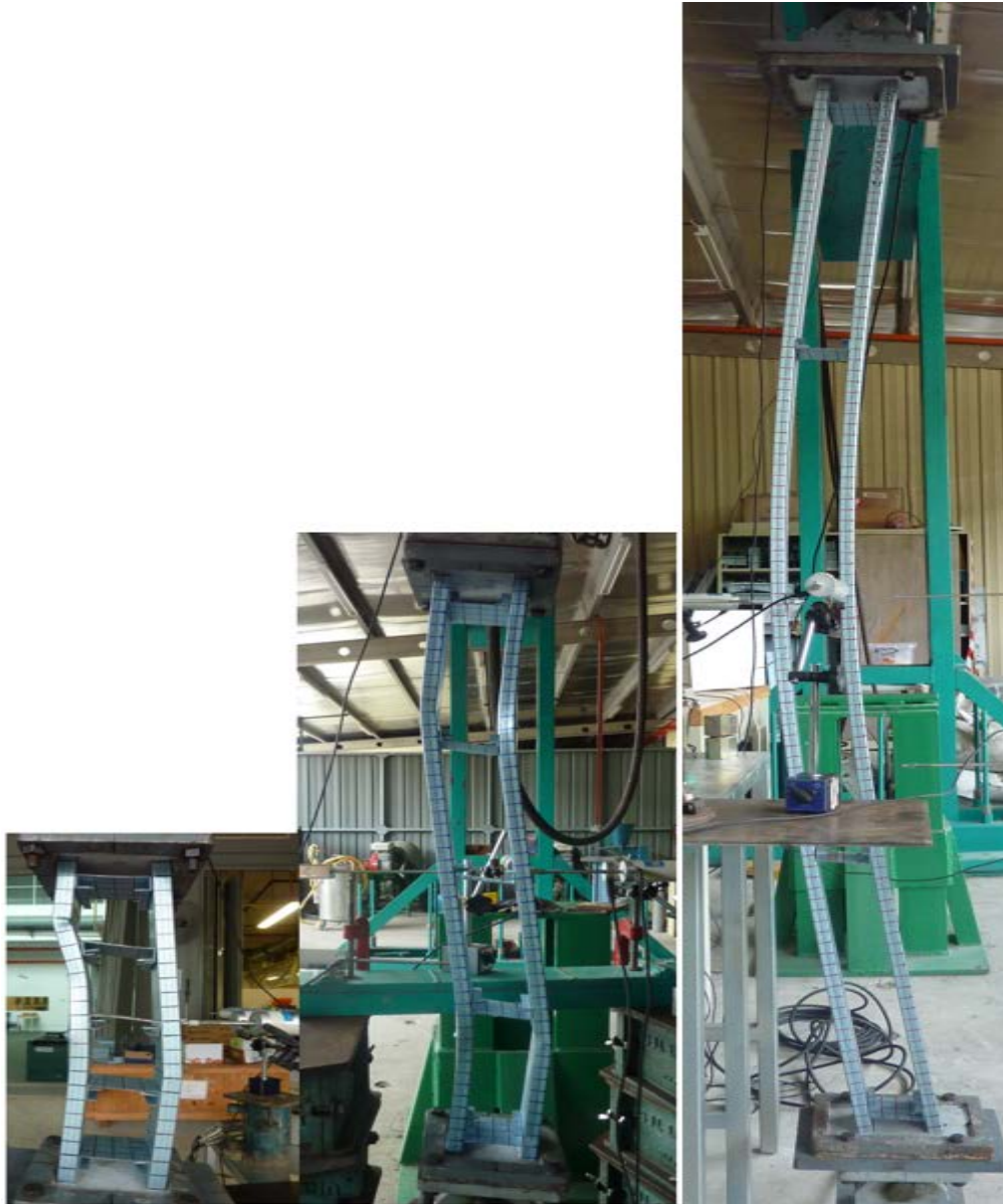
(a) GBU75-S100-L500 (Mode-A) (b) GBU75-S225-L1000 (Mode-A) (c) GBU75-S475-L2000 (Mode-B) Figure 10: Photograph of short, intermediate and slender columns at failure
