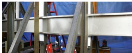
Fig. 9 Obvious distortional deformation in compression flange at peak load of member B-1
