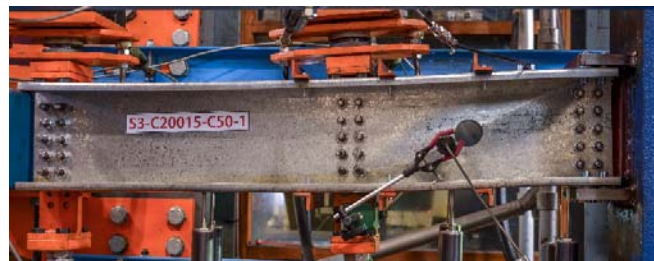
(c) Circular hole with a 50 mm diameter
