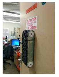
**Rise-Rover**: a wall-climbing robot to carry heavy NDT instruments (>50lb) for visual and contact-based inspection.
