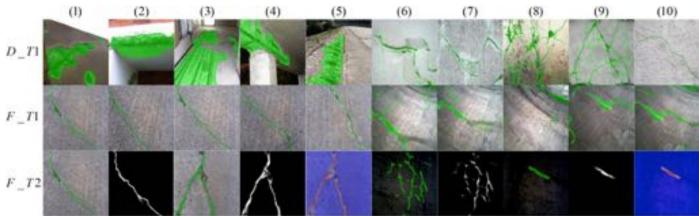
Develop InspectionNET for surface flaw detection and measurement.
