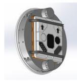
**GPR-Rovers**: custom designed wall-climbing robots to carry GSSI's ground penetrating radar (GPR) for detecting subsurface defects, locating rebar and pipes.
