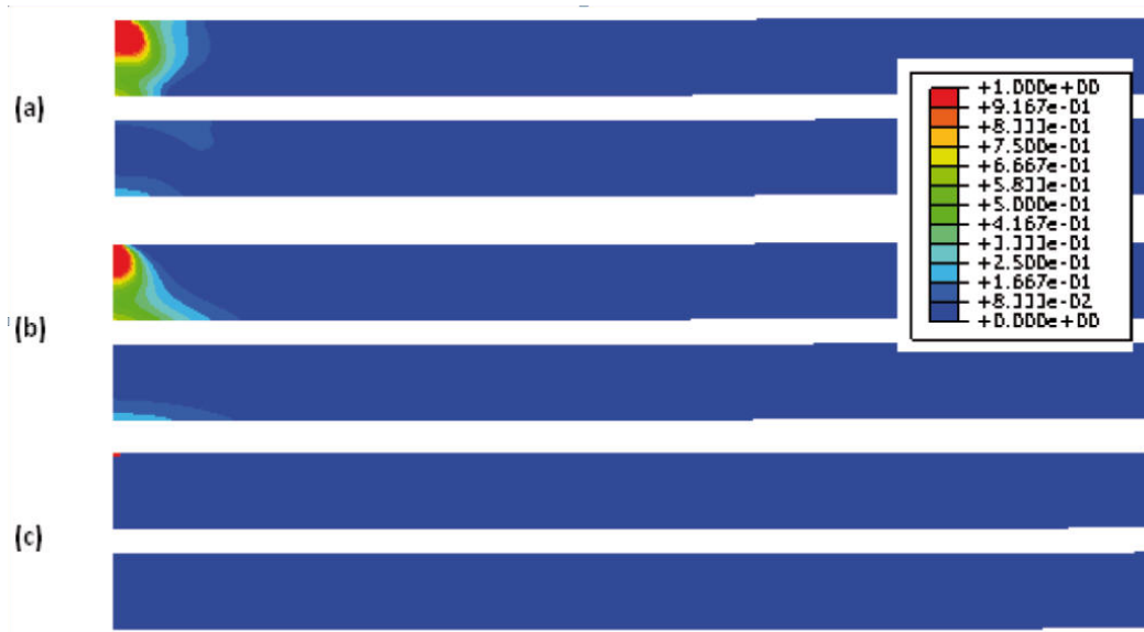
Figure 5. Contour plots of damage in laminated glass at 3.4 ms after impact for large missile with round end configuration: (a) web-shaped damage D_{11} ; (b) star-shaped damage D_{33} ; (c) shear damage D_{12} .
