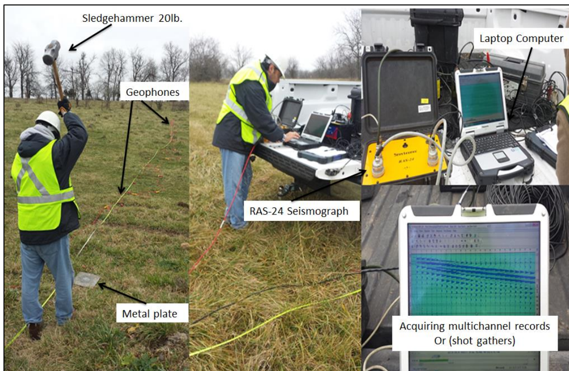
Figure 4.3. Active MASW data acquisition.
