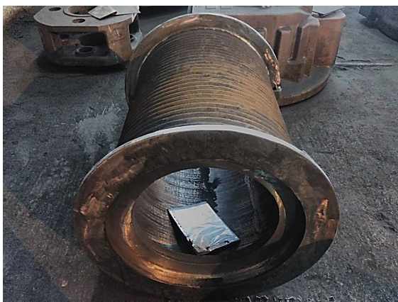
Fig. 1. Rope drum cast
