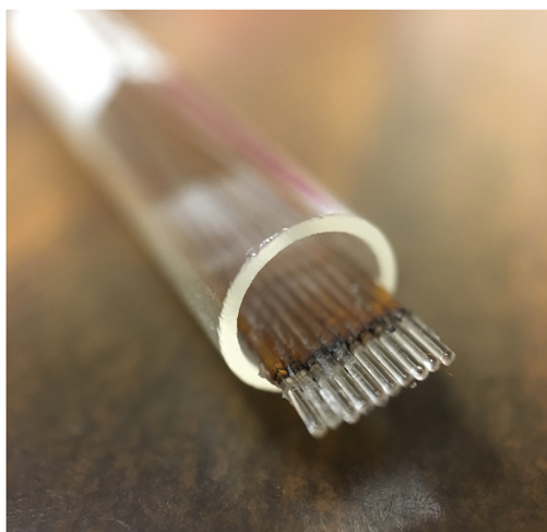
FIG. 1. Photograph of a 10-capillary Gradient CapPack contained in a 5-mm NMR sample tube.
