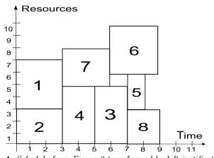
Fig. 4. Schedule from Figure 3 transformed by left justification
