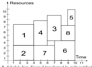
Fig. 3. Schedule from Figure 2 transformed by right justification
