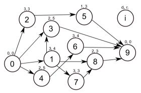
Fig. 1. Example of project in Activity-On-Node representation
