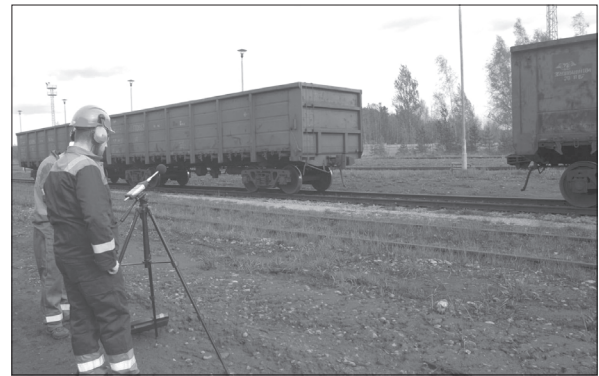
Fig. 1. Registration of the collision of train cars
